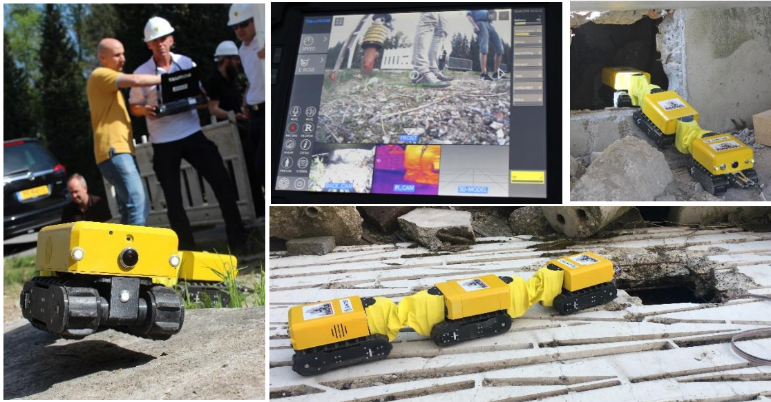
The robot and its rugged graphical user interface
