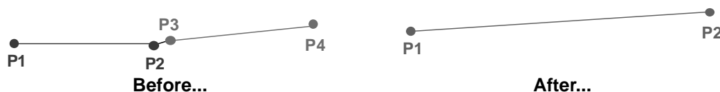
Figure 3-15: Removal of unnecessary corners when two successive line segments are likely to be parallel and the distance between them is lower than 50cm
