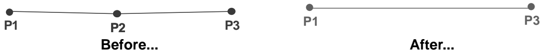
Figure 3-7: Removal of unnecessary corners when points that create with the previous and following point form the same line segment or an extremely large angle
