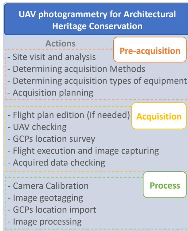
Figure 4 UAV Photogrammetry for Architectural Heritage Survey Research Activity
