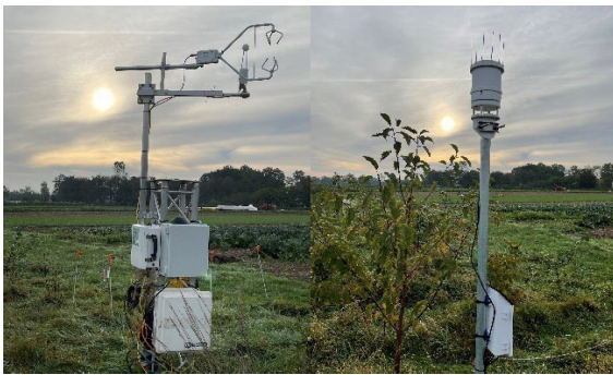
Eddy Covariance and energy balance Station (left) and automatic weather station (right).
